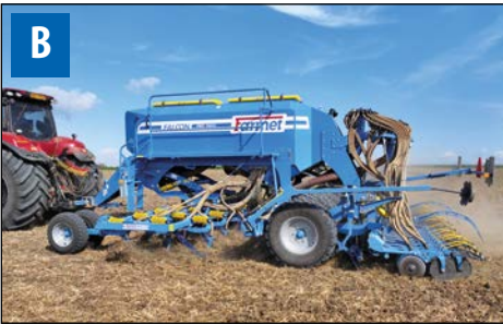
Sowing of rape with deep cultivating and fertiliser application.
