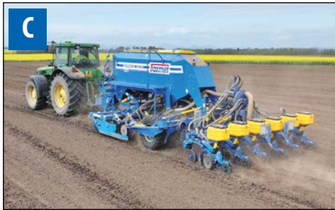
Precision sowing of corn and fertiliser application.
