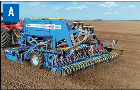
Sowing of cereals into narrow lines with possibility of fertilisation under the heel.
