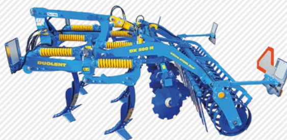
Version with hydraulic setting the working depth
