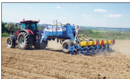
Mounted seed drill for sowing wide-row crops.
