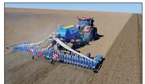
Wide working width sowing section for narrow-row crops sowing.
