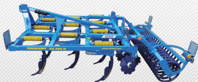
Version with mechanical setting the working depth
