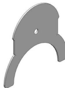
Picture 32 Gauge for assessing the wear of K80
