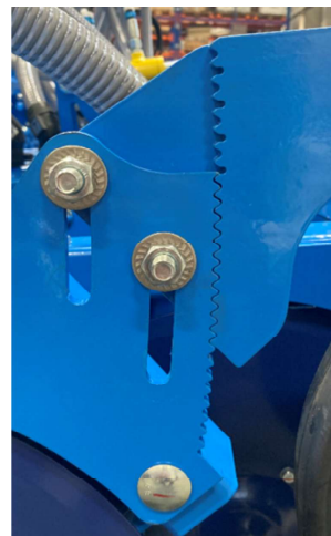
Depth of sowing coulter by 4 cm.
