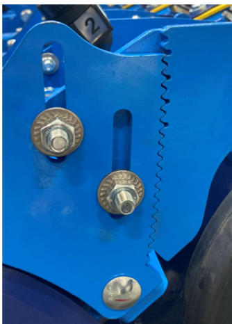
Depth of sowing coulter by 1 cm.
