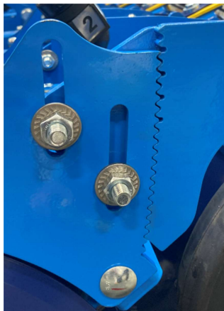
Depth of sowing coulter by 1 cm.
