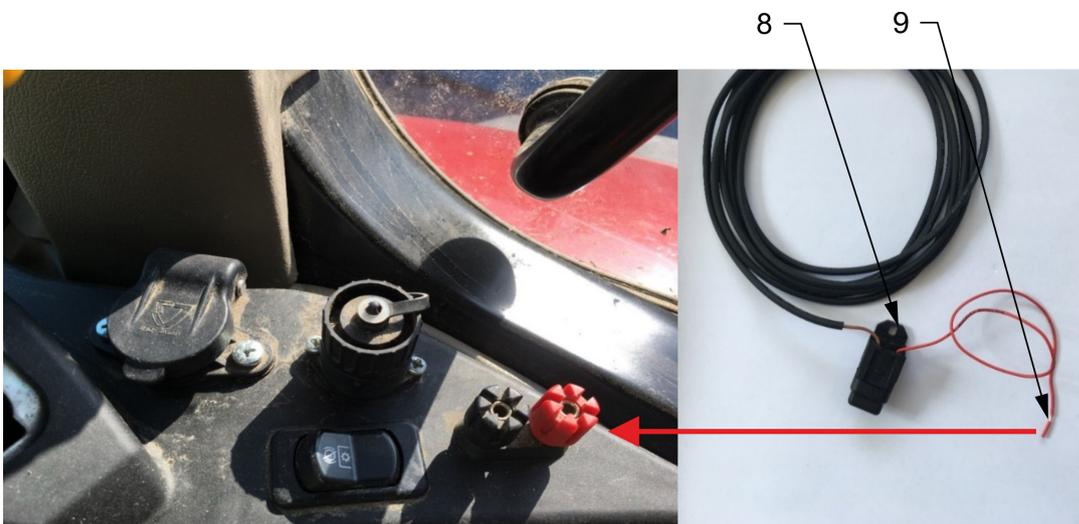
**8.4.3.2 Connecting the machine via the ISOBUS socket of the tractor + Müller terminal**
