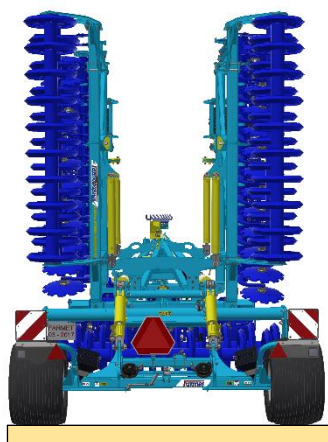
Picture 11 – Machine position for unfolding
